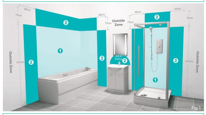
All installations must comply with guidelines which are based on a zonal concept Fig.1. This concept must be followed to ensure the safe installation. These regulations apply to domestic installations only. Installations must be made in accordance with the current IEE wiring regulations and relevant building regulations.
